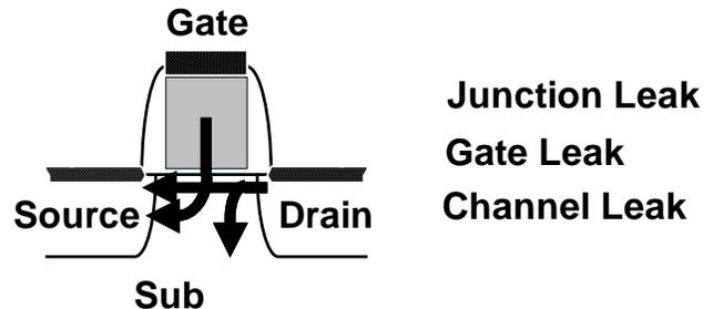
FIGURE 2 LEAKAGE-CURRENT PATHS OF A MOS TRANSISTOR
