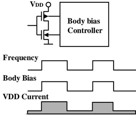
FIGURE 3 CONCEPT OF BODY BIAS CONTROL METHOD
