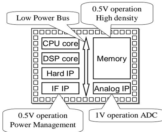
FIGURE 1 STRUCTURE OF SoC IN 90NM TECHNOLOGY
