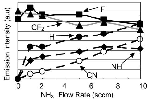
Fig. 5 OES intensity vs NH<sub>3</sub> flow rate.
