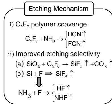
Fig. 3 Mechanism of NH<sub>3</sub> adding effect.
