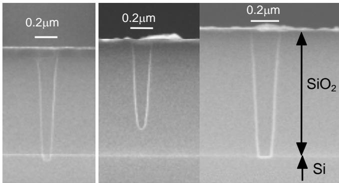
(a) O<sub>2</sub> added (b) H<sub>2</sub> added (c) NH<sub>3</sub> added
