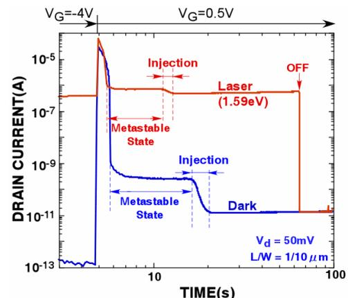
Fig. 2 Temporal changes in the drain current measured at  $V_g = 0.5V$  under irradiation of 780nm (1.59eV) light and dark condition after complete discharging of the Si-QDs floating gate at  $V_g = -4V$ .
