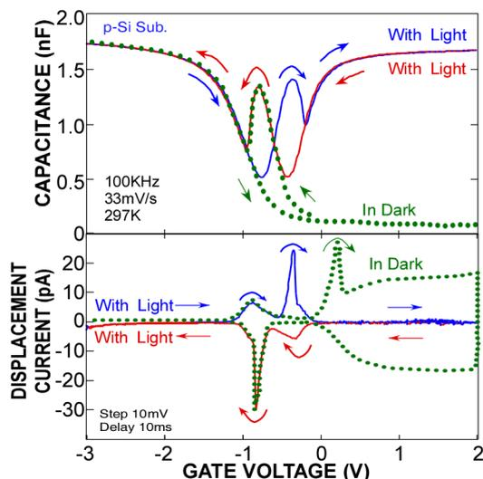
Fig. 1 100kHz capacitance-voltage and displacement current-voltage characteristics of an Al-gate MOS capacitor with a Si-QDs floating gate measured at room temperature in dark and under illumination of cold light in the wavelength region of 400-800nm.
