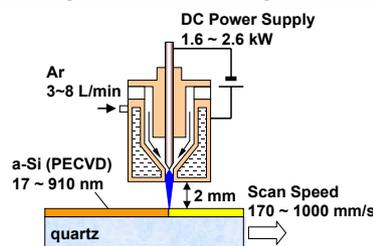
Fig. 6. Schematic diagram of experimental setup for annealing of a-Si film by thermal plasma jet.
