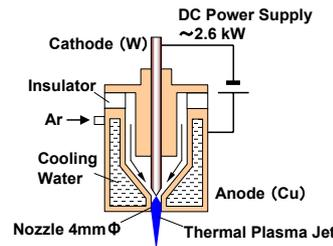
Fig. 2. Schematic diagram of thermal plasma source.
