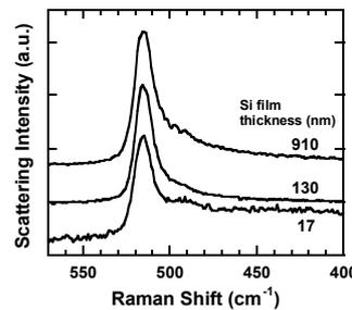
Fig. 12. Raman scattering spectra of crystallized Si films with the thickness ranging from 17 ~ 910 nm. The broad peaks in lower wave number regime seen in 17 nm film is the signal from quartz substrate. Both thin and thick a-Si films have been crystallized. This is because the thermal diffusion length of this annealing technique is much larger than the film thickness.
