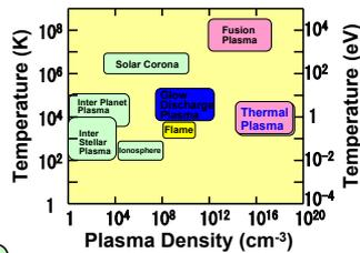
Fig. 1. Mapping of various plasmas based on the density and the temperature.
