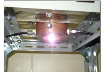
Fig. 3. Photograph of thermal plasma jet generated by atmospheric pressure discharge.
