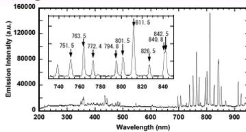
Fig. 4. Optical emission spectrum of thermal plasma jet. Most of the significant lines are identified to be emission from Ar atoms as indicated in the inset. From the Boltzmann's plot of the Ar lines, the temperature of the plasma was roughly estimated to be 8,300K.
