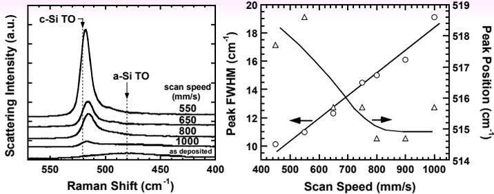
Fig. 8. Raman scattering spectra of Si films before and after the annealing. 80nm-thick a-Si films are crystallized by the thermal plasma jet.
