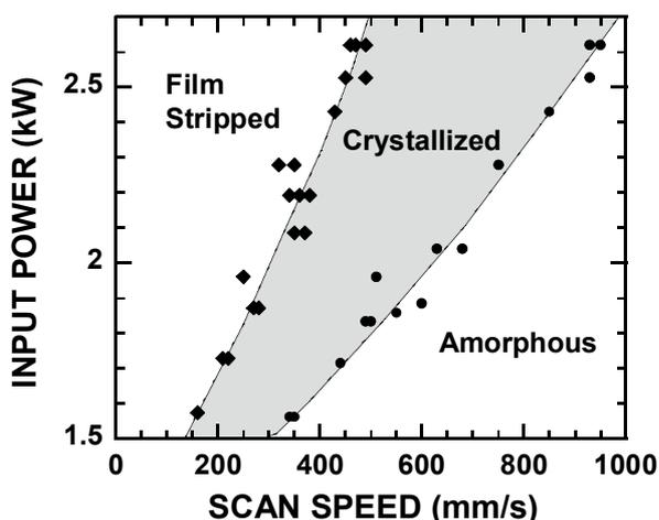
Fig. 3. Conditions of input power to the plasma source and scanning speed for the crystallization of a-Si films.
