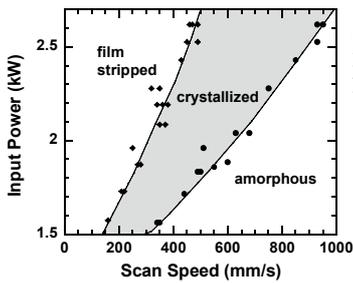
Fig. 11. Crystallization condition of input power and scan speed. a-Si film is crystallized over a wide annealing condition. No de-hydrogenation is required, the film stripping was facilitated with a decrease in the scanning speed down to a certain value
