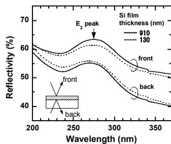
Fig. 13. UV reflectivity spectra of crystallized Si films obtained from top and backside of the substrate. Spectra obtained from 130 and 910 nm thick films are compared. Clear  $E_2$  peak are observed from both samples. The Si film is completely crystallized to the bottom interface independent of film thickness.
