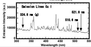
Fig. 5. Identification of emission lines from Cu in thermal plasma jet. No emission lines from Cu was observed in the optical emission spectrum of thermal plasma jet.
