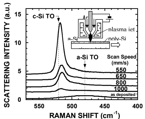
Fig. 2. Schematic diagram of thermal plasma jet annealing of Si films on glass (inset) and Raman scattering spectra of 80 nm thick Si films annealed by thermal plasma jet.
