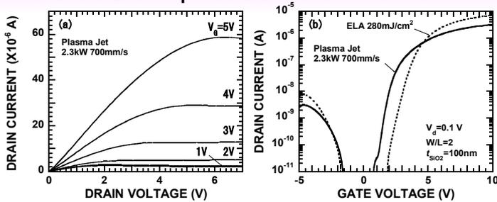
Fig. 14. Output (a) and transfer (b) characteristics of TFT fabricated by thermal plasma crystallization technique. For comparison, ELA TFT is also fabricated on the same substrate.
