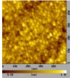
Fig. 10. AFM image of a Si film crystallized by thermal plasma jet. ( $V_{Si}$ : 20 nm, input power: 2.57 kW, scan speed: 600 mm/s, Ar flow rate: 10.5 l/min) roughness: 3.5 nm (RMS: 0.53 nm) grain size: 20~30 nm
