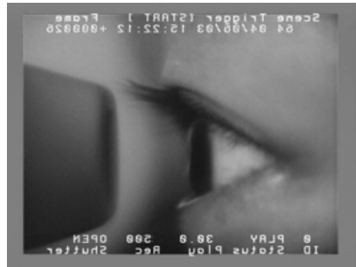
Fig. 1 Eye deformation due to an air jet.
