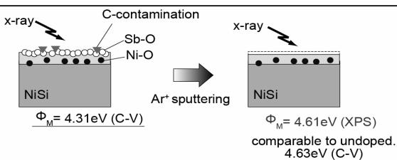
Sb-O signal was disappeared after Ar<sup>+</sup> sputtering necessary for workfunction evaluation.
