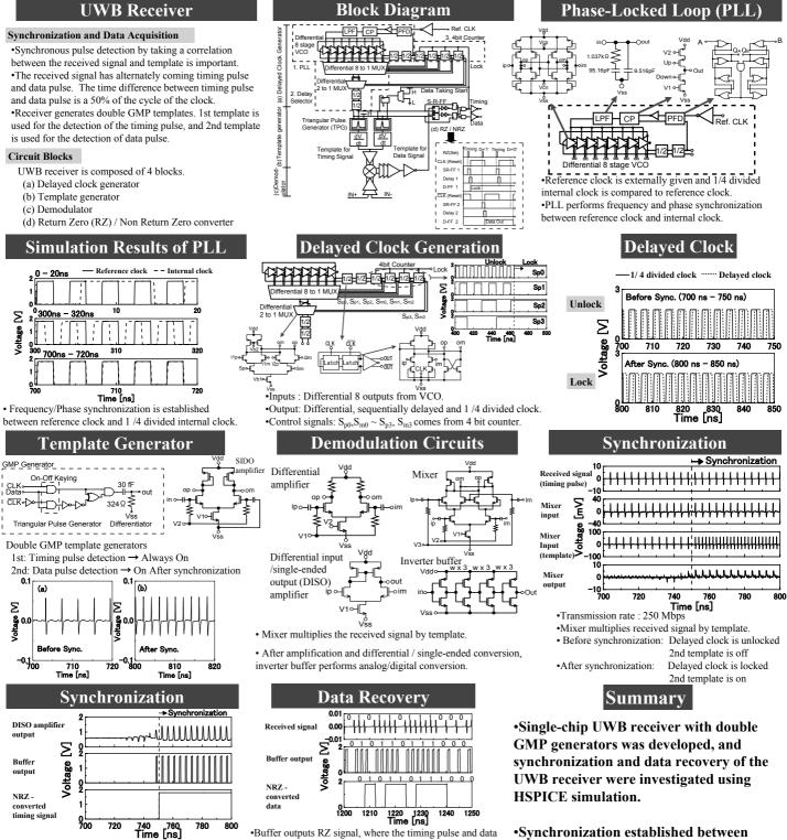
•The synchronization establishes around 750 ns. •NRZ-converted timing signal is used as a flag of the establishment of synchronization, i.e., the signal locks delayed clock.
